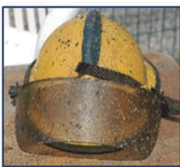
Figure 12: An example of surface contamination
